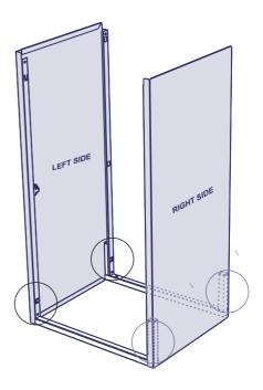
1 - With the end of **F3**, smash the safety claw, locking the **FRAMES** to the **LEFT SIDE** and **RIGHT SIDE**.
